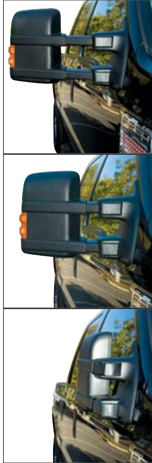
Ford's electric folding mirrors require less space than conventional mirrors when folded, and offer a clear view of the side of the trailer when they're extended for towing.
